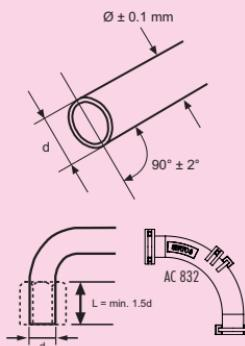
For the union is a **straight, unblemished tube end** needed with a **length 'L'** of at least  $1.5d$ . If necessary, use bend clip AC 832
