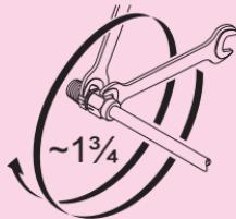
Tighten down the union nut approx.  **$1\frac{3}{4}$  rotations** using an open ended spanner. Hold the nipple with a second wrench.
