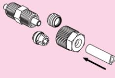
**Insert the tube** into the union **as far as the stop**. Verify that the hose has been pushed through the entire clamping ring.
